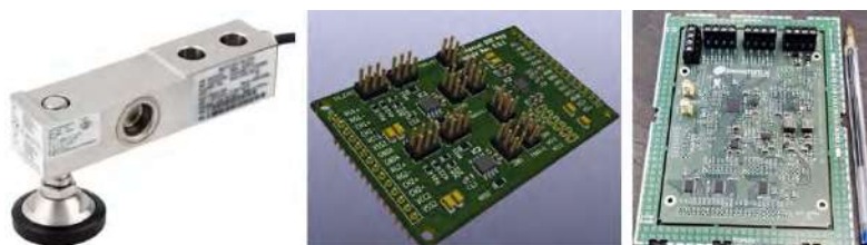
Figure 3. Shear beam load cell and custom designed and built PCBs for project needs.
